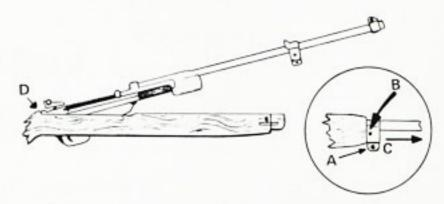
Draw operating spring guide slightly to rear until it is disengaged from operating slide, and then pull to right and forward and withdraw guide and spring from well in receiver.
