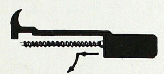
Draw recoil spring guide slightly to rear until it is disengaged from operating slide, and then pull to right and forward and withdraw guide and spring from well in receiver.
