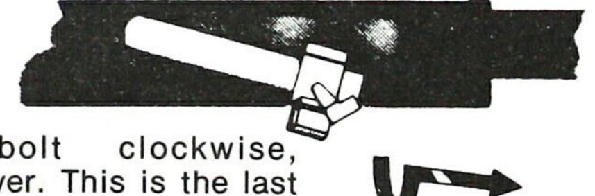
way in receiver. Then rotate bolt clockwise, and lift it up and right to remove from receiver. This is the last step in field stripping.
